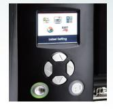
Color TFT LCD and operation panel for easy and intuitive operation
