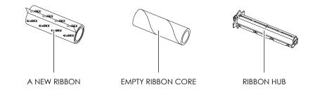
1. Attach the ribbon to the empty ribbon core with the adhesive strip at the end of the ribbon.
