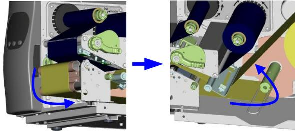
29. Replace the printer cover to complete the installation.
