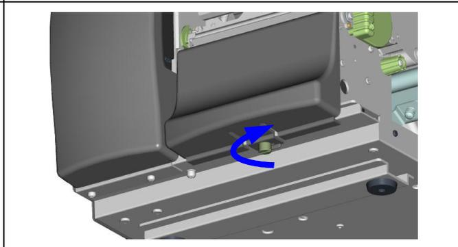
2. Remove the two screws securing the tear-off plate, then remove the tear-off plate.
