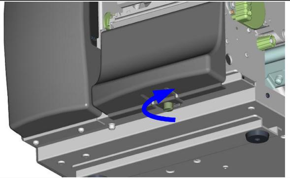
3. Mount the rewriter guide on the print mechanism and secure it with screws.
