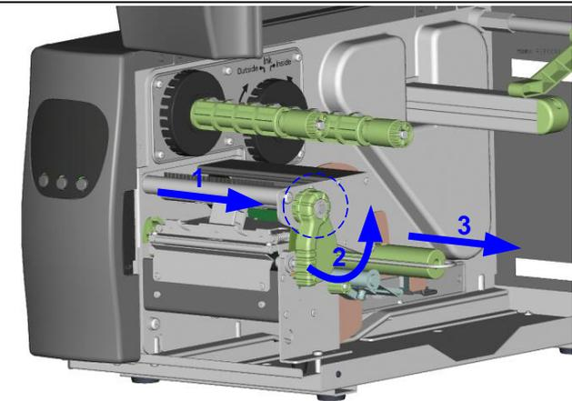
6. Now load the label roll into the printer.
