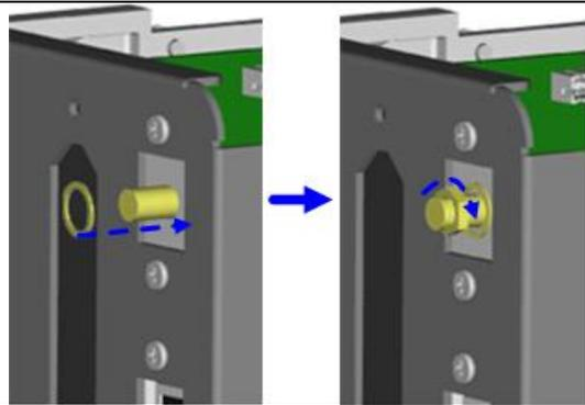
22. Screw the antenna onto the antenna connector. You can now adjust the angle of the antenna as required.
