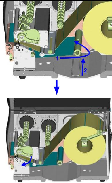
13. Close the printer cover to complete installation of the dispenser.
