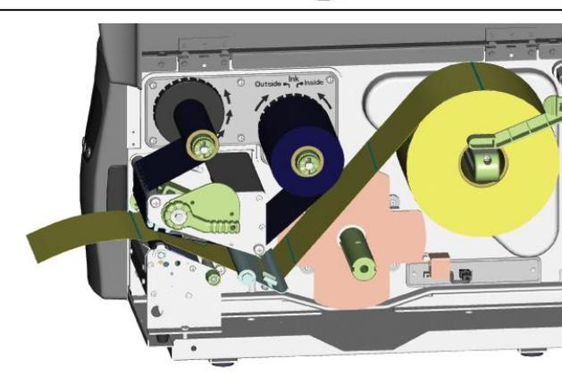
7. Strip a few labels off the label liner (approx. 400 mm). Then pass the label liner through the print mechanism and from the bottom up onto the rewriter.
