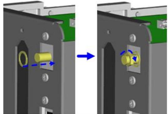
11. Turn the Antenna according to the direction as arrow showed to mount it on the Antenna Connection Wire. The angle of Antenna can be adjusted if needed.
