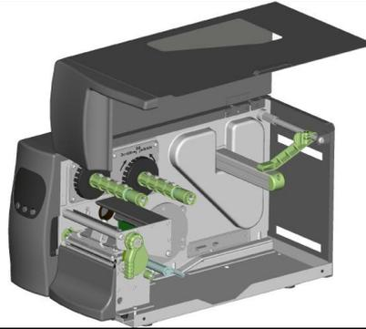
2. Pull out the print head release lever as shown in the illustration (1) and turn it anticlockwise to a top right position (2).
